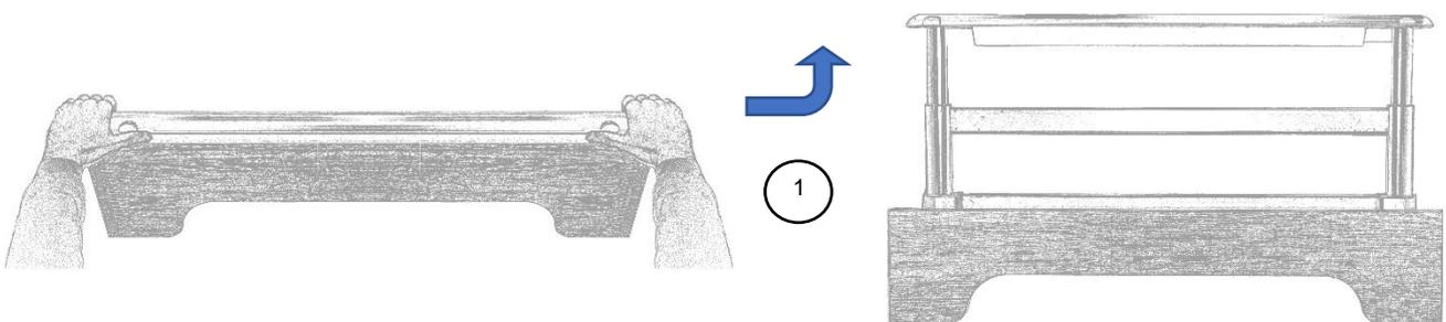
② Check that the side rail is locked by trying to fold it without using the unlocking buttons.
