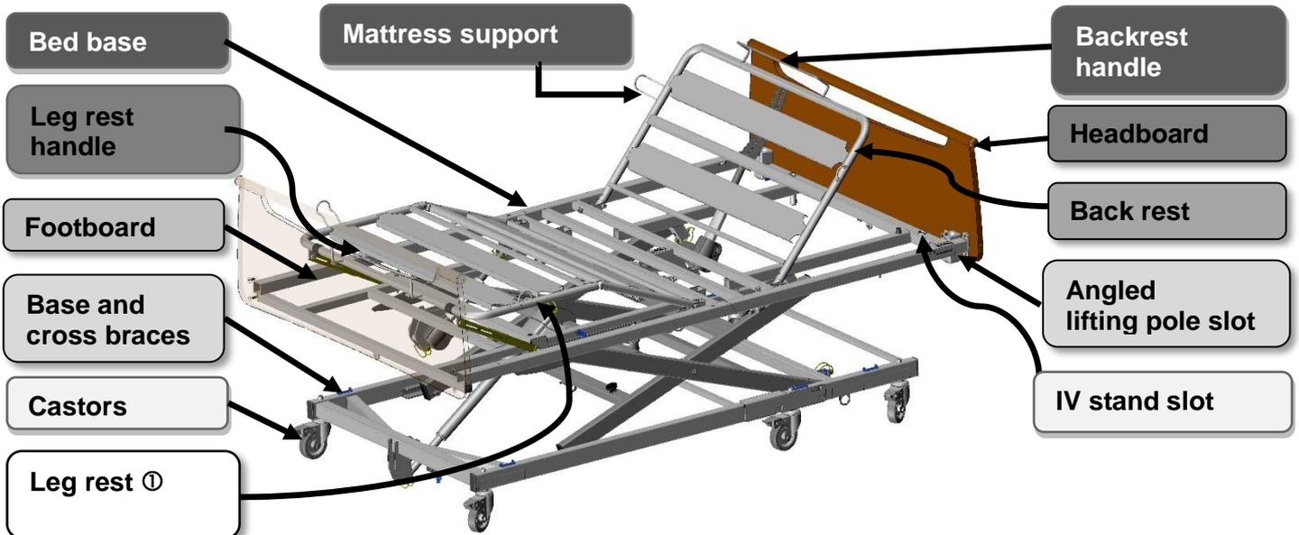
① Manual crank or electric folding leg rest depending on version.
