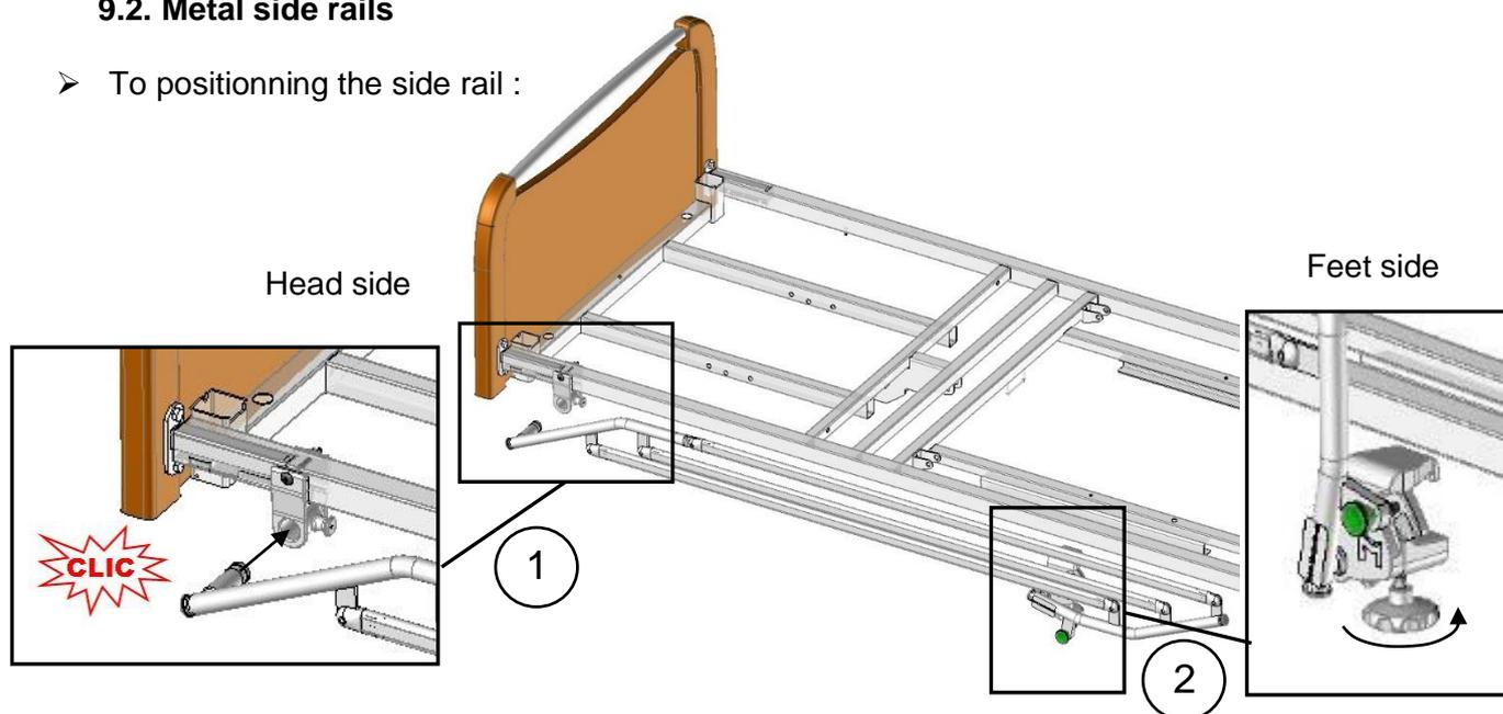
① Insert amount of the side rail folded in the grip jaw on the head side of the bed to hear “CLIC”.
