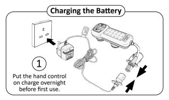
We recommend that the hand control is left continuously on charge when the Archimedes is not in use, as a matter of routine.
